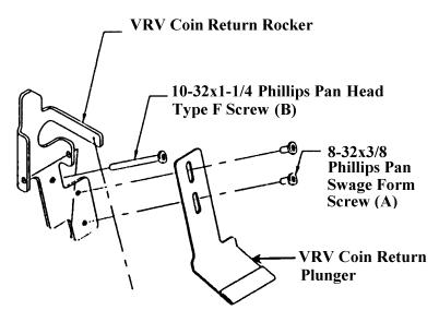
This Dixie-Narco vender is equipped with an adjustable VRV Coin Return Plunger. The VRV Coin Return Plunger is adjustable to enhance its use with different coin mechanisms.
